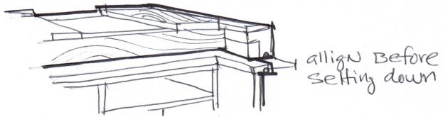
5. Remove crate carefully. Remove the employee side 2x6 wood by unscrewing top supports. Make one person hold one end while unscrewing supports. Remove the end support then lift up the rest of the crate. Push counter top to front leaving no space between the countertop and the cabinets.
