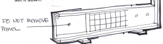
Make sure the bottom of countertop and top of cabinets are clear of any material that can block the installation when you set it down
