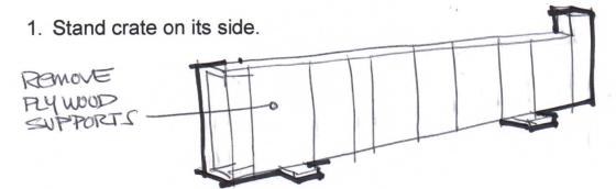
Remove plywood supports to expose the bottom of the counter top. DO NOT remove the 1/2" plywood panel that supports the cold topping cutout. Flip it down carefully and get ready to set it on the service counter cabinets. You need at least 4 people to set it down.
