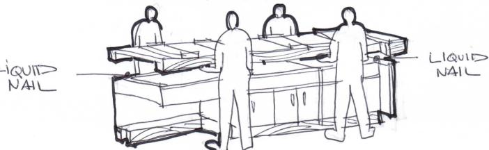
4. Align the countertop extension (8" extension on the POS side) with the side panel and lower it carefully. Make sure the countertop is set perfectly before going to the next step.
