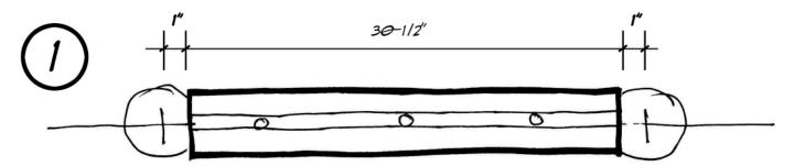
LOCATE THE POSITION OF THE GPB THEN DRAW A CENTER LINE. SET THE GPB IN THE CENTER THEN MARK 3 HOLES FOR THE WEDGE BOLTS THEN MARK I" FROM BOTH ENDS (OF BASE SHOE) FOR THE CENTER OF THE CORE POCKET.
